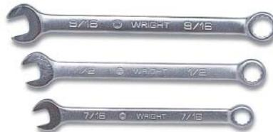
**Combination wrench**—has both box and open-end heads. Both ends are for the same size bolt.
