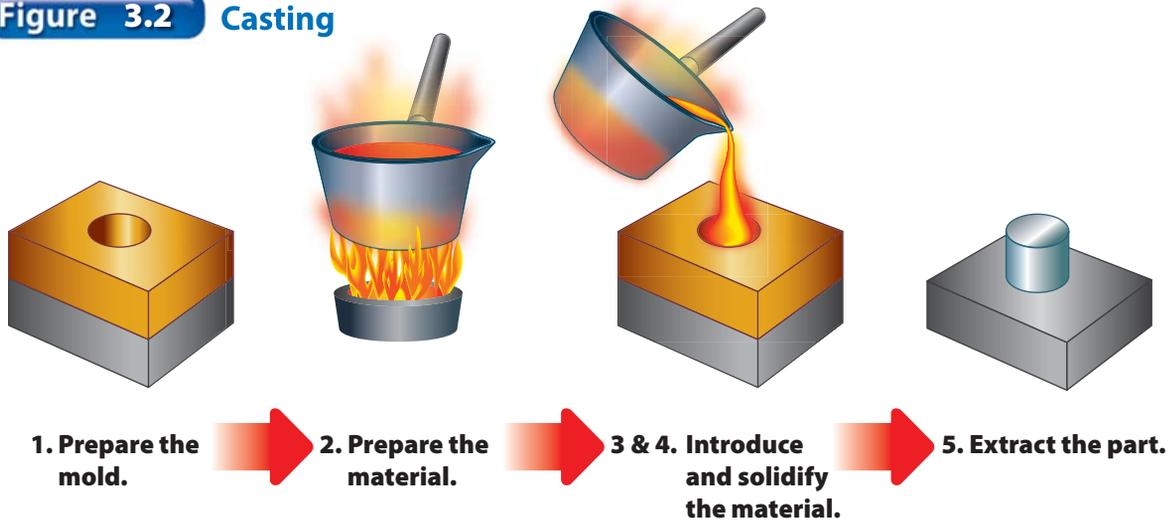
**Liquid to Solid** Molten metal, glass, clay, or plastic material takes on the shape of the mold as it cools. *What items do you use at home or school that might have been made by casting?*
