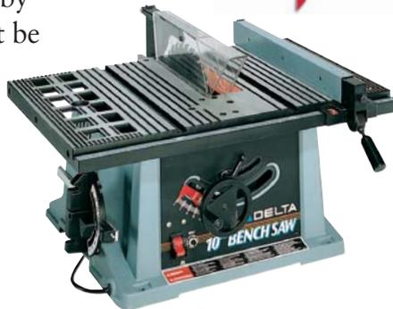
**Table saw**—the most commonly used saw. Its size is determined by the diameter of the largest blade it can use.
