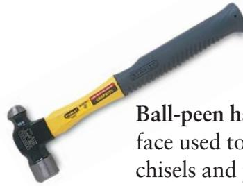
**Ball-peen hammer**—one face used to strike cold chisels and punches; the other face for shaping soft metal
